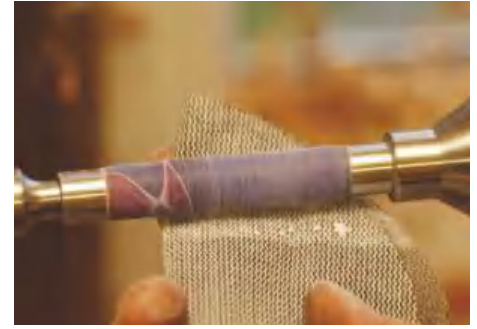
▲ Pic.9 Abrading with fine dry abrasives gets the barrels clean and uniform
